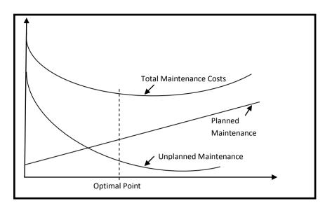
Figure 1: Trade-off between Planned and Unplanned Maintenance.
