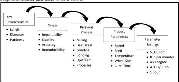
Figure 2: Key Characteristic to Process Parameters
